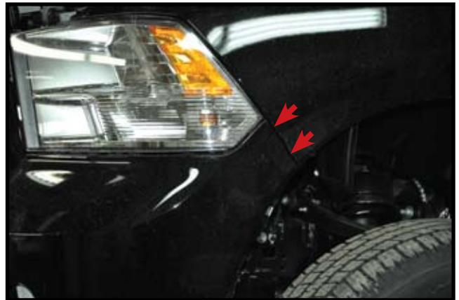
5. Remove fascia by pulling down to release plastics studs then forward.
