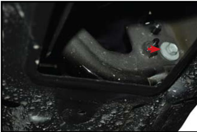
3. Inside of each inspection hole remove one bolt that attaches the fascia to front fender.
