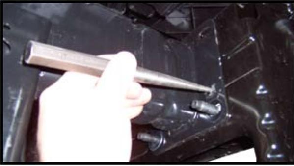
7. Flatten raised tab with a hammer and punch.
