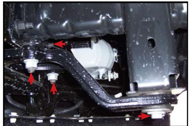
6. If equipped with tow hooks remove three bolts that hold the hook and remove the three nuts from the bumper and remove brackets. **NOTE:** The hook, brackets and the three bolts will not be reused.
