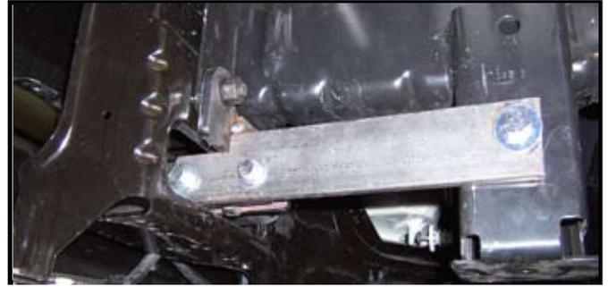
10. Attach rear brace on back of each pull pod using two 3/8" x 1-1/2" bolts, two 3/8" washer and two 3/8" lock washer connecting it to frame with one 7/16" x 5-1/2" bolt ,one 7/16 lock washer and one 7/16" flat washer and 7/16" nut and tighten all bolts. Use blue **LOCTITE** on bolts and tighten all bolts according to chart on front page.
