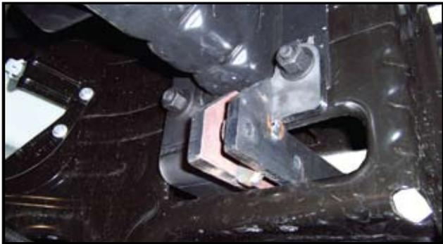
9. Place pull pod on the 3 bolts studs and replace 3 nuts leaving nuts loose Repeat steps 3, 4 ,5 and 6 for opposite side.
