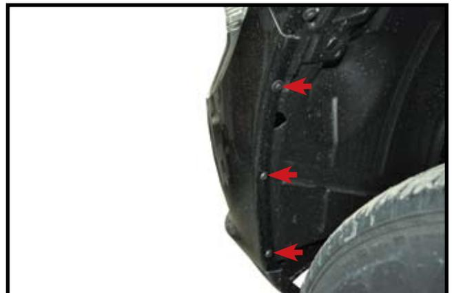
1. Remove one screw and two plastic screw fasteners from each wheel well in front of tire.
