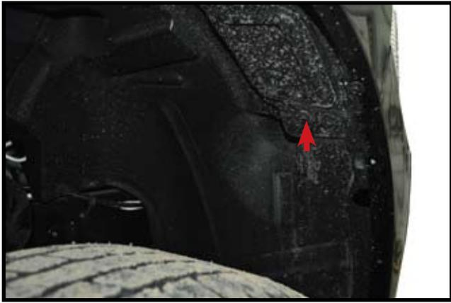
2. Remove one plastic push fastener from each inspection flap in front portion of each wheel well.
