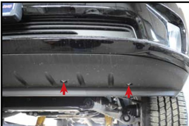
4. Remove two screws from each side from bottom of fascia.
