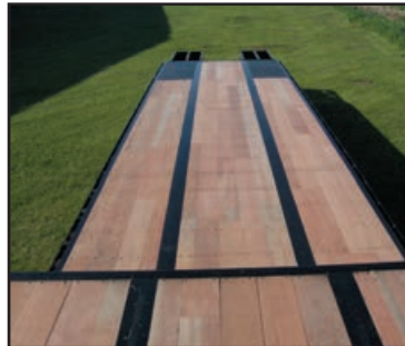
Apitong Flooring (screwed to every cross member)
