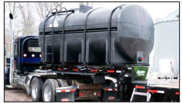
Black plastic liquid tanks eliminate light from reaching the interior contents preventing algae and microbes growth
