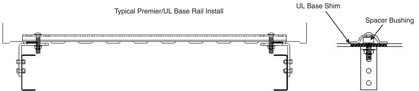
End view showing spacer spanning from flange to flange under the base rail. Place rail spacer bushing as shown.
