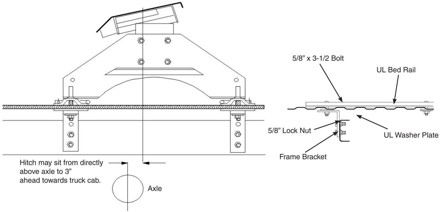
**IMPORTANT NOTICE:** This installation may require different frame brackets for the various truck models. This kit does not contain any frame brackets for this reason. Frame specific installation instructions are available at our website [www.towdemco.com](http://www.towdemco.com) or by calling (800)543-3626. Optional brackets are shown below.
