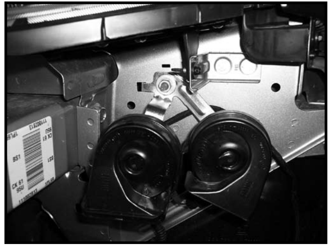
6. Remove one screw and unplug horn and set aside.
