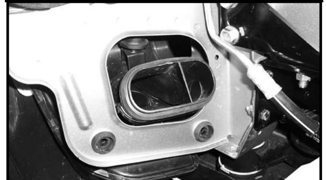
8. Remove one screw and remove air box tube. Push air box back and then down so inlet is out of way.
