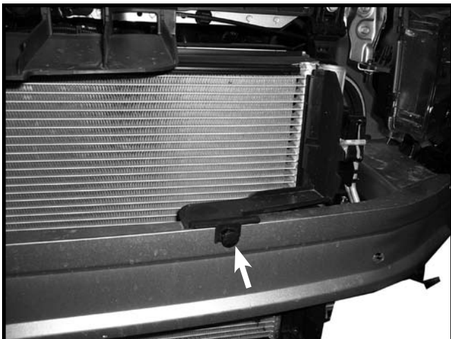
5. Remove one plastic push fastener from each air deflector and remove. NOTE: Drivers side shown.
