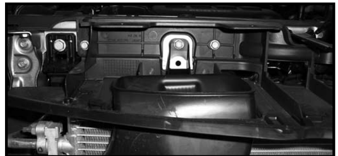
7. Remove plastic fastener for cooling line. Remove two bolts from each side of bumper they will not be reused.
